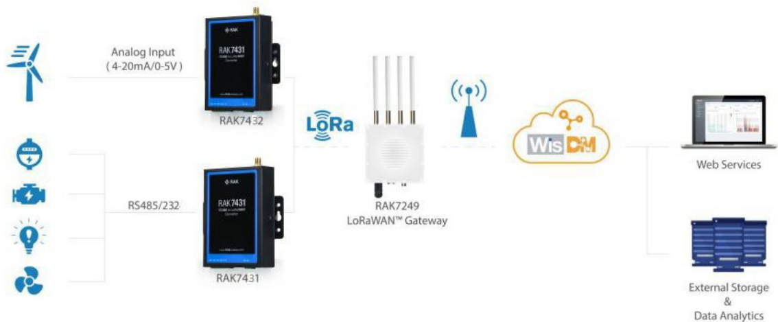
Figure 1 | RS485 to LoRaWAN™ network structure
