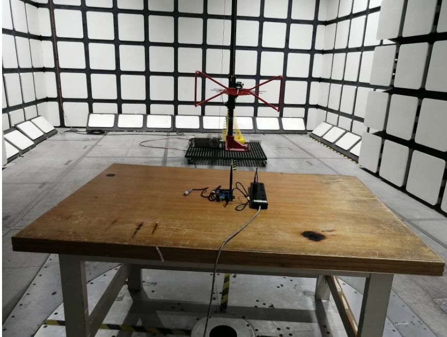
Radiated Emissions View (Below 1 GHz)
