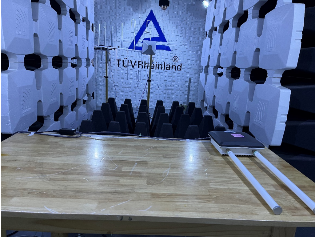
Photograph 3: Set-up for Radiated Emissions, above 1GHz
