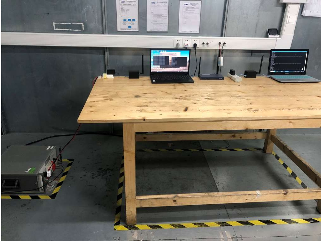
Photograph 1: Set-up for Conducted Emissions, AC Mains
