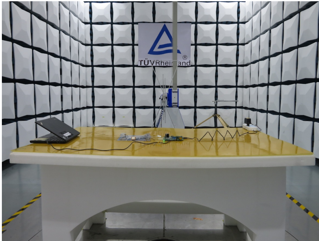
Photograph 1: Set-up for Radiated Spurious Emission, Below 1GHz
