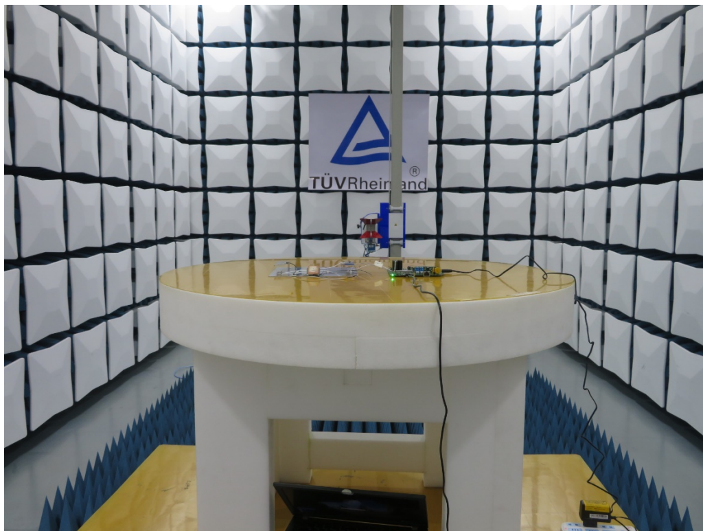
Photograph 2: Set-up for Radiated Spurious Emission, Above 1GHz
