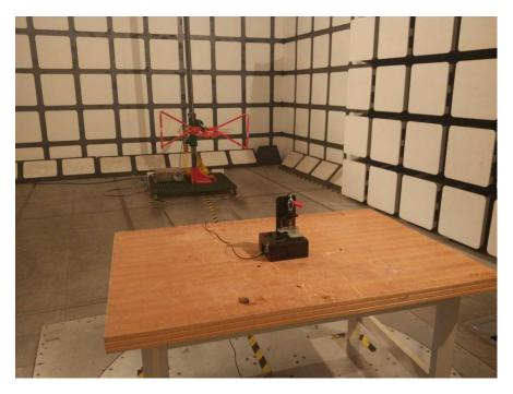
Radiated Emissions View – Onboard Antenna (Below 1 GHz)
