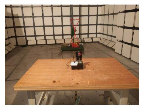
Radiated Emissions View – External Antenna (Below 1 GHz)
