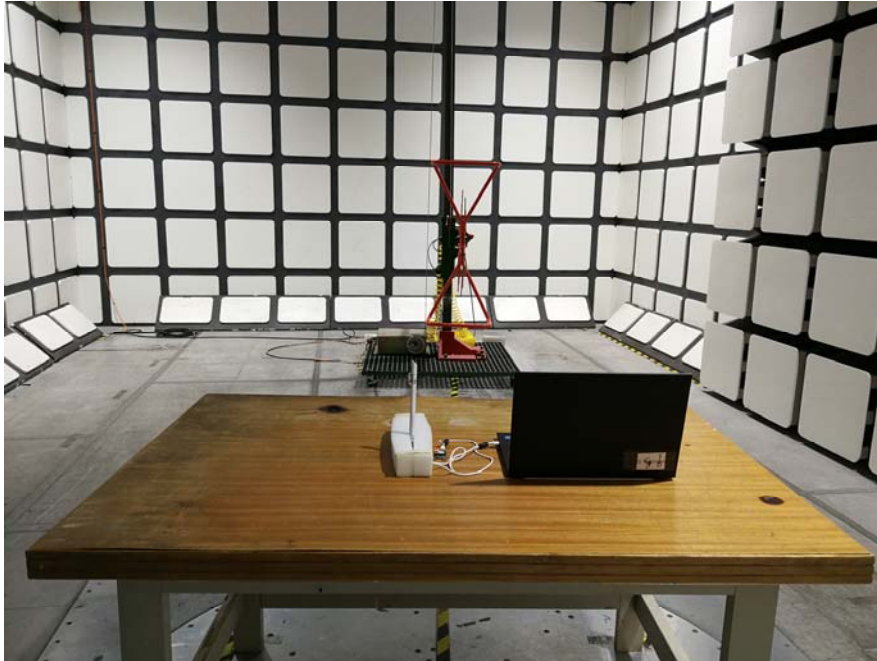
Radiated Emissions View (Below 1 GHz)
