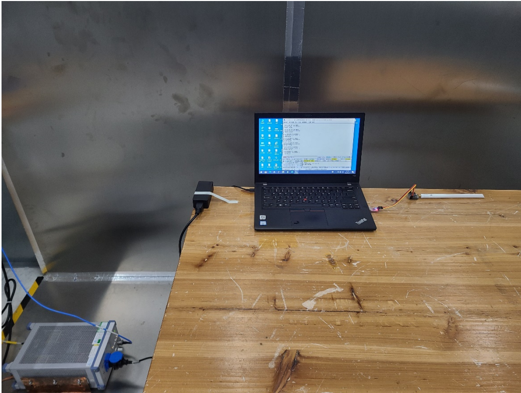
Photograph 3: Set-up for Conducted Emission on AC mains
