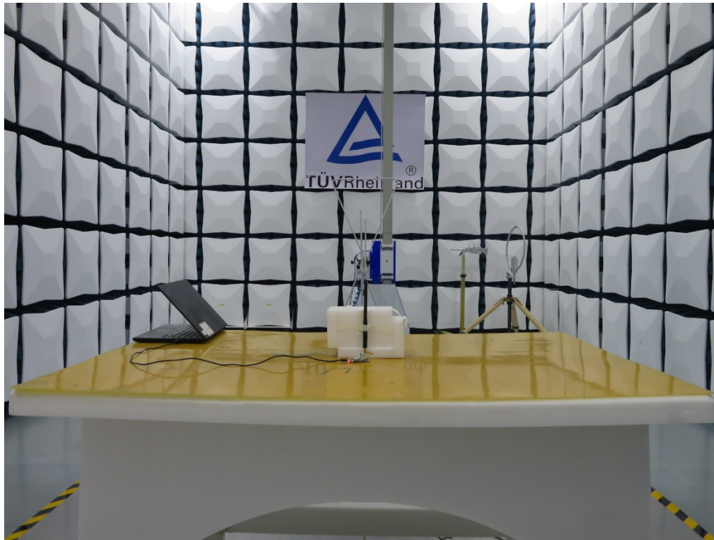
Photograph 1: Set-up for Radiated Spurious Emission, Below 1GHz
