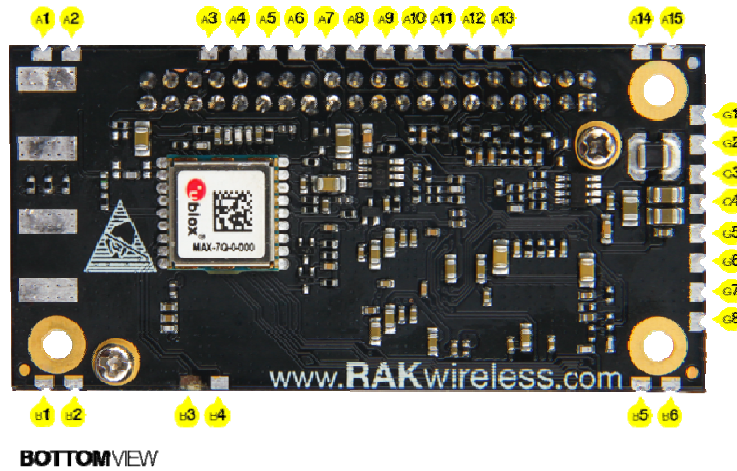
Figure 2 | RAK2245 Pin Definition
