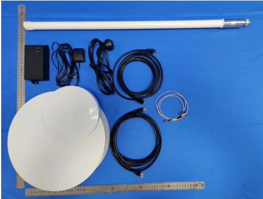
EUT with fiberglass Antenna (5.1dBi)
