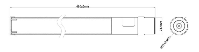
Figure 3: RAKARG19 mechanical specifications
