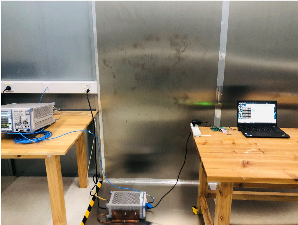
Photograph 3: Set-up for Conducted Emission on AC Mains
