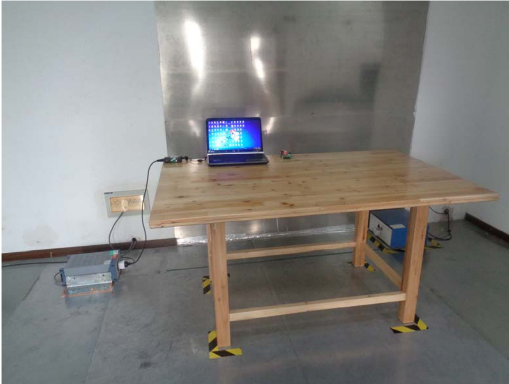
Conducted Emissions Test Setup – Front View
