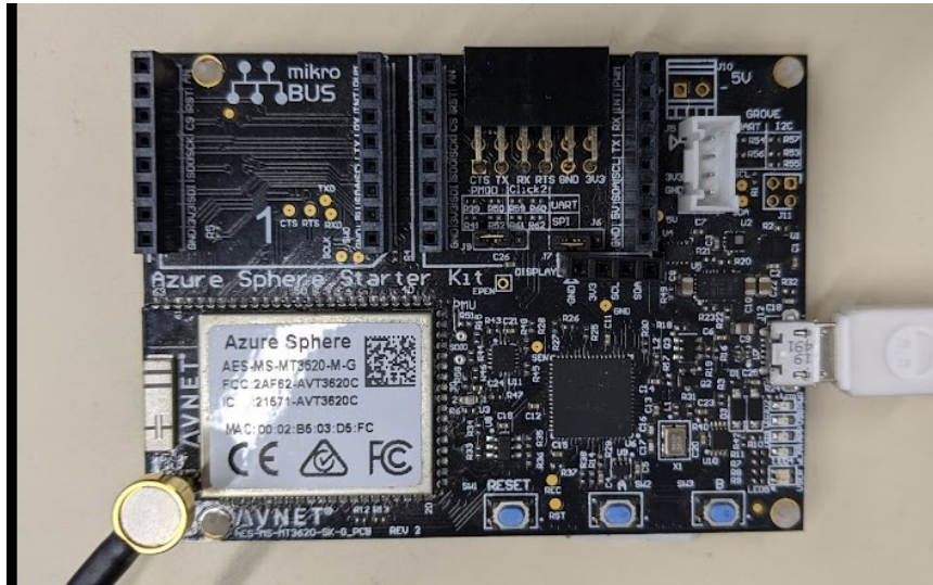
Figure 1 – Test setup showing antenna, temporary antenna connector and USB connection
