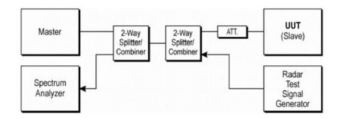
Figure 3-1. Conducted Test Setup for DFS
