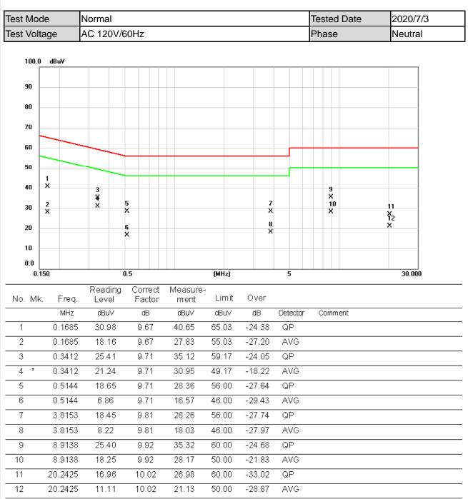
(1) Measurement Value = Reading Level + Correct Factor.
