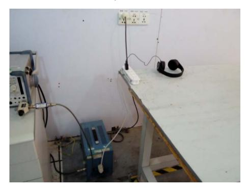
Radiated spurious emissions Test Setup(below 1GHz)
