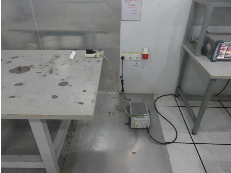
Photo of Conducted Emission Measurement
