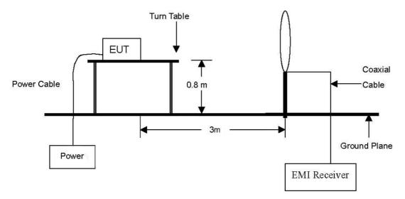
The diagram below shows the test setup that is utilized to make the measurements for emission from 30 Mz to 1  $\mathbb{G}_{\mathbb{Z}}$ .
