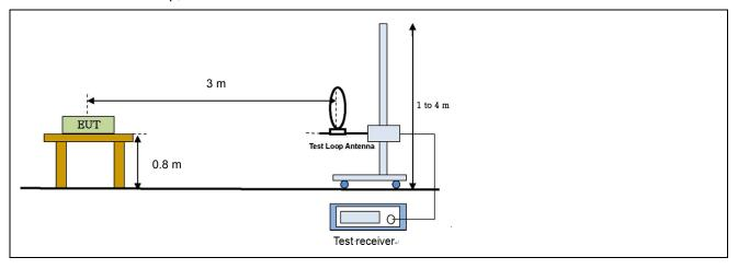
Radiated emission setup, Below 1 000 MHz
