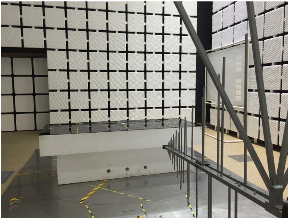
Radiated RF measurement (30 MHz - 1 GHz)
