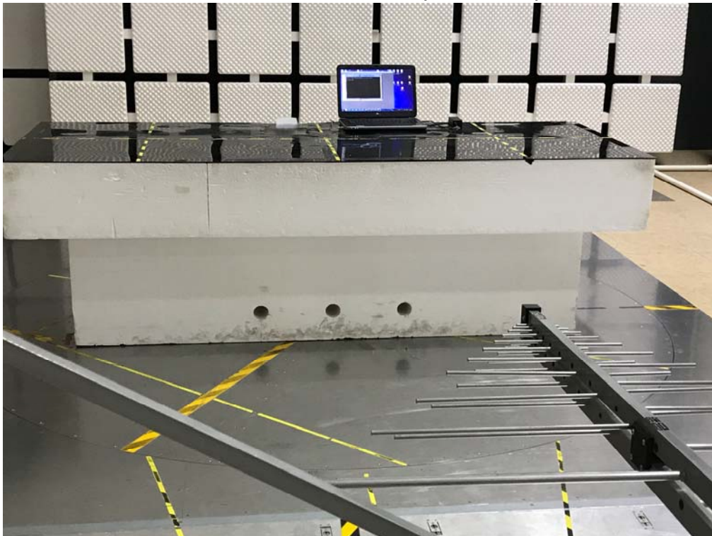
Radiated RF measurement (30 MHz - 1 GHz)
