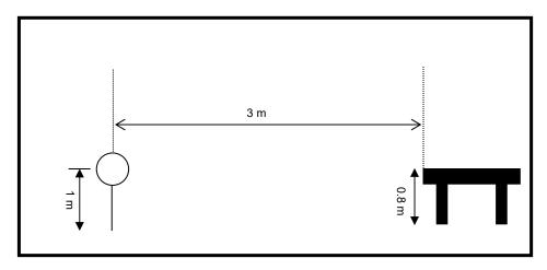
Radiated emission setup, below 1 000 MHz
