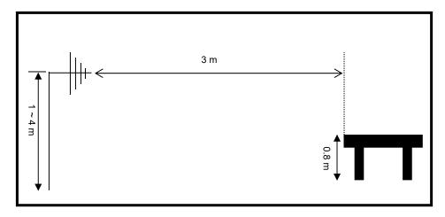
Radiated emission setup, above 1 GHz
