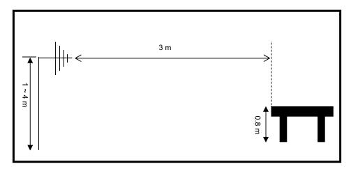
Radiated emission setup, above 1 GHz
