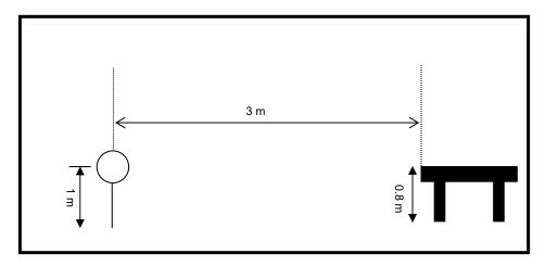
Radiated emission setup, below 1 000 MHz
