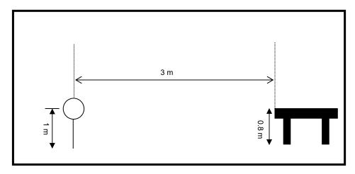
Radiated emission setup, below 1 000 MHz
