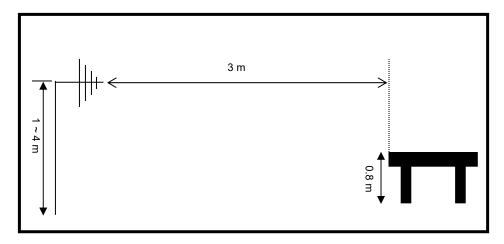
Radiated emission setup, above 1 GHz
