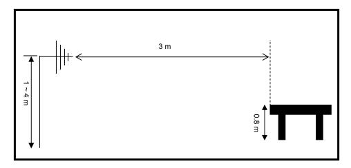
Radiated emission setup, above 1 GHz
