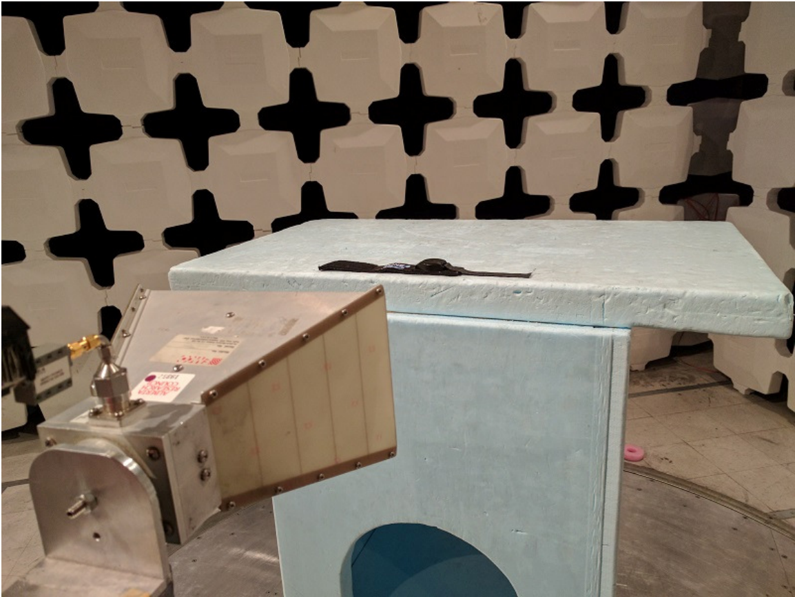
Figure 6 – Radiated Emissions, Pre-scan, 18 GHz to 26.5 GHz:
