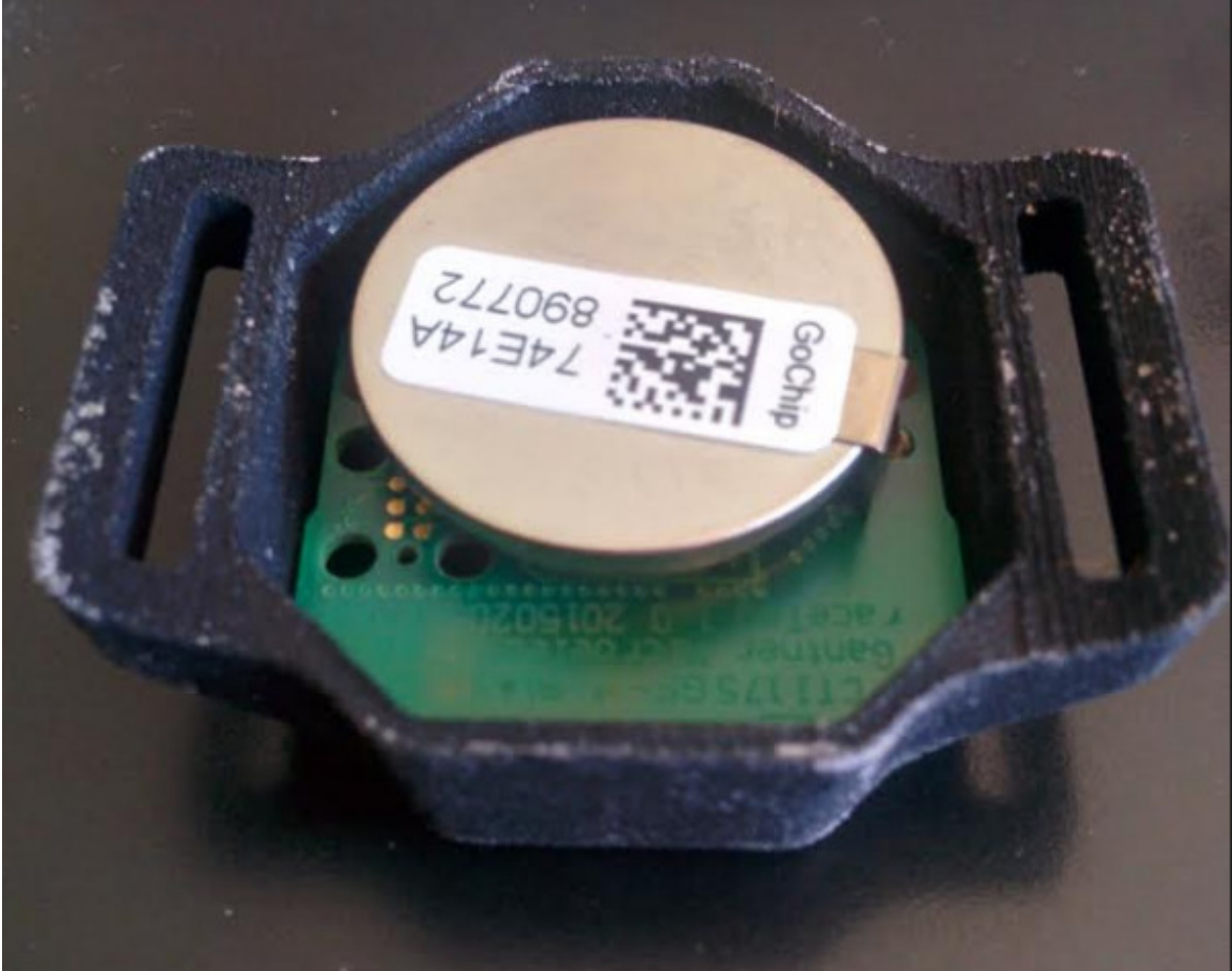
Figure 4: After urethane potting
