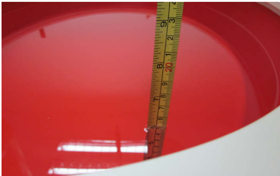
Figure 4.4: Liquid depth in the Flat Phantom
