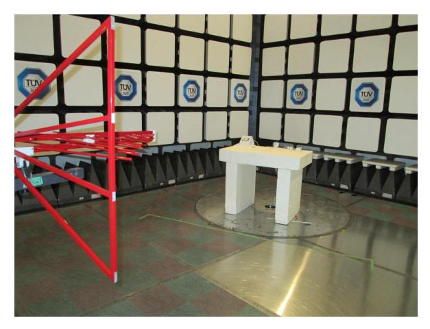
Test setup photo 2 Radiated measurements, 30 MHz – 1 GHz
