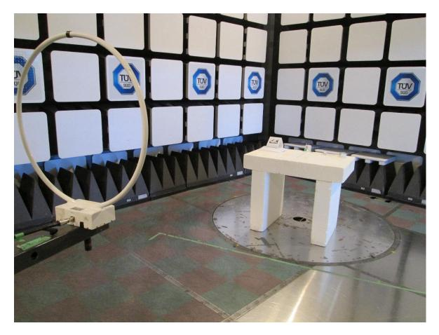
Test setup photo 1 Radiated measurements, 9 kHz – 30 MHz
