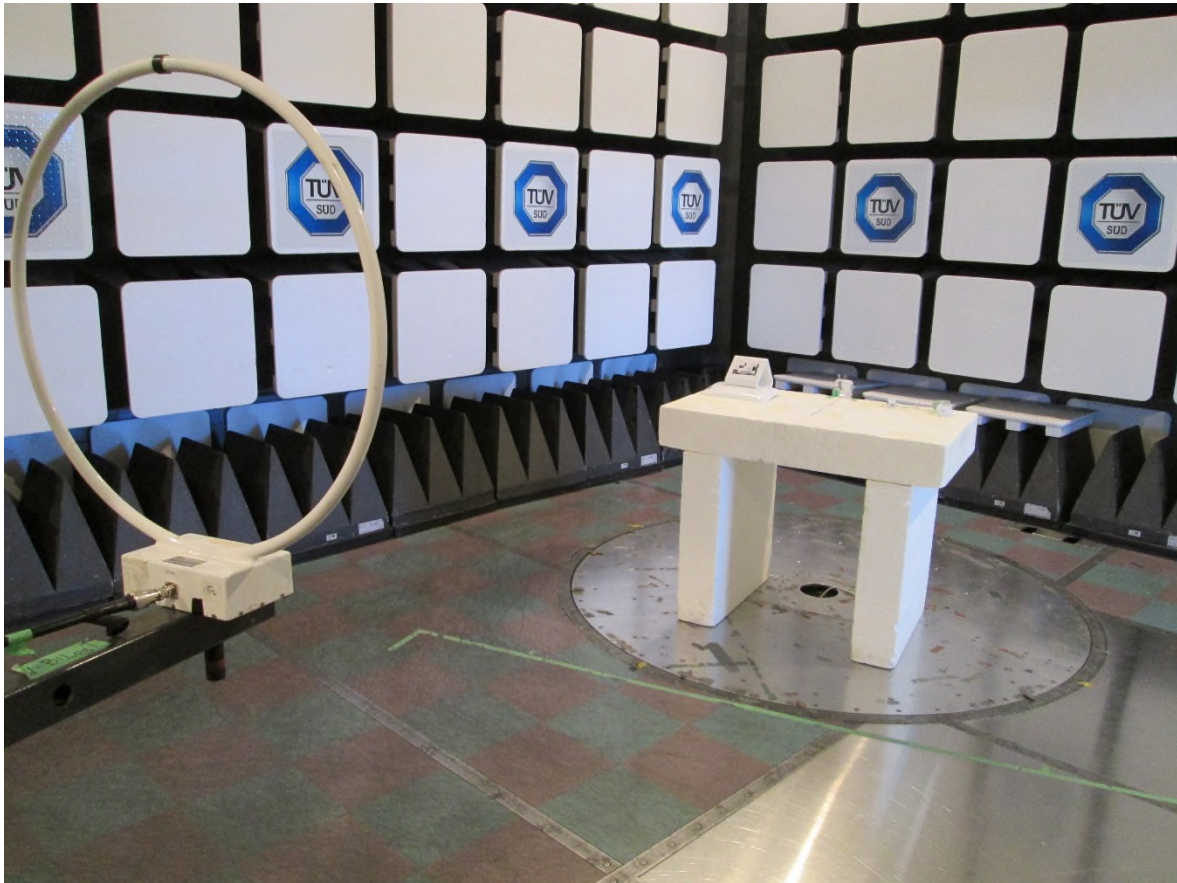
Test setup photo 1 Radiated measurements, 9 kHz – 30 MHz
