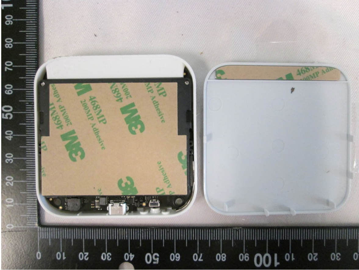
EUT – Internal view 1 Back cover removed.
