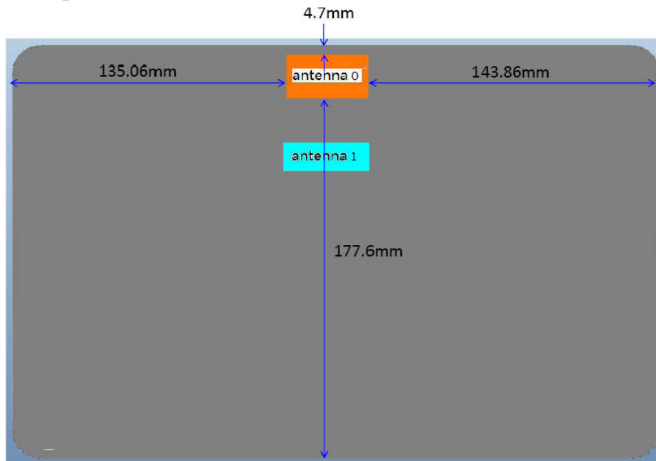
(Antenna 0)Front of the screen view
