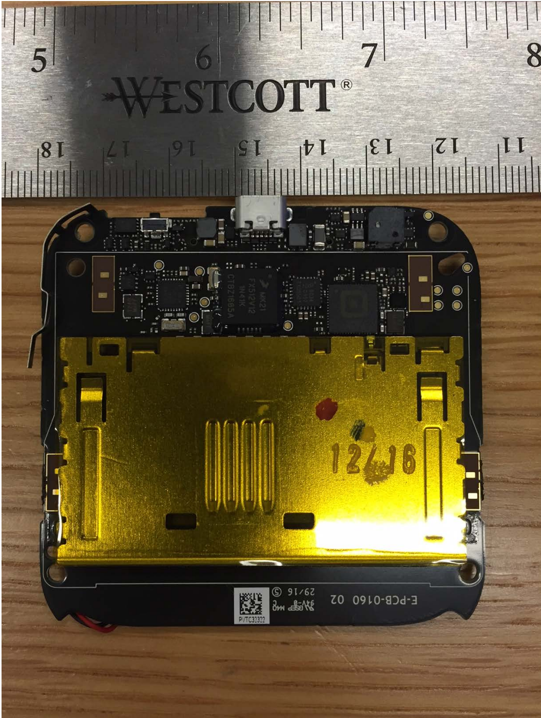
EUT - Internal view 3 PCB, side 1, cage removed
