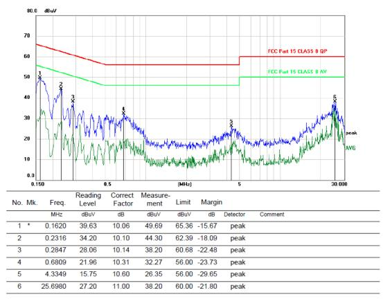
Note: Measurement=Reading Level+Correc Factor. Factor=(LISN or ISN or PLC or Current Probe)Factor+Cable
