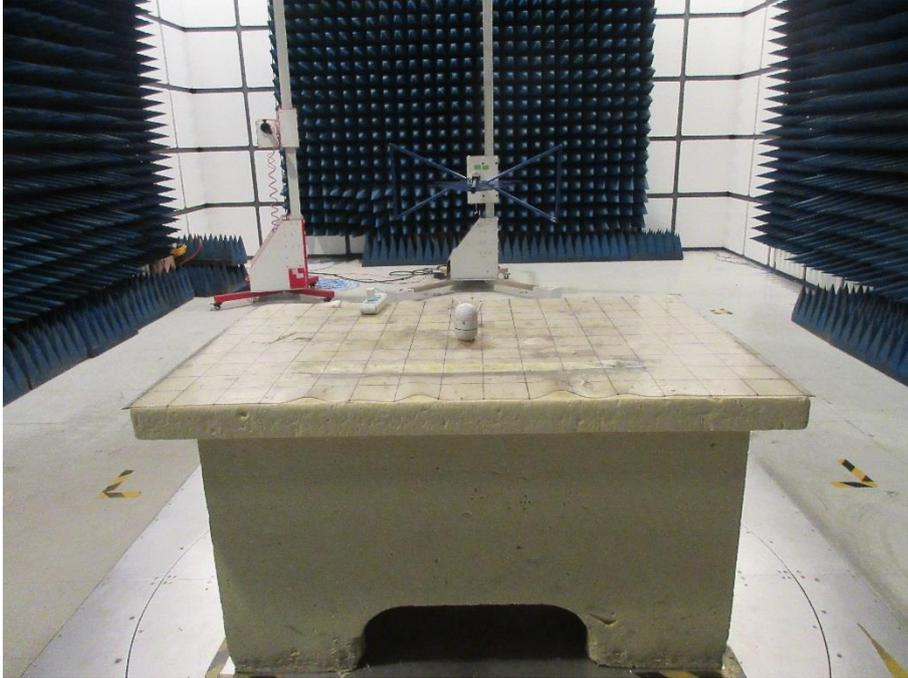
Radiated SPURIOUS EMISSION SET-UP PHOTOS, 1GHz ~ 25GHz
