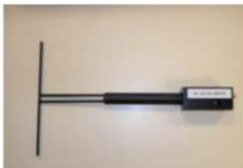
Figure 1 – Satimo COMOSAR Validation Dipole
