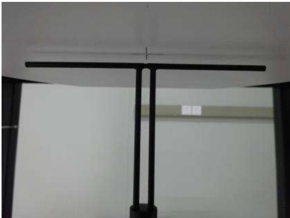
Photo of Dipole Setup
