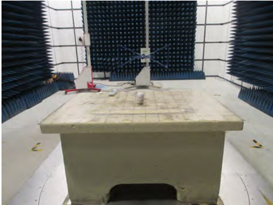
Radiated SPURIOUS EMISSION SET-UP PHOTOS, 30MHz ~ 1GHz
