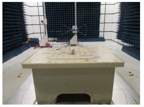
Radiated SPURIOUS EMISSION SET-UP PHOTOS, 30MHz ~ 1GHz
