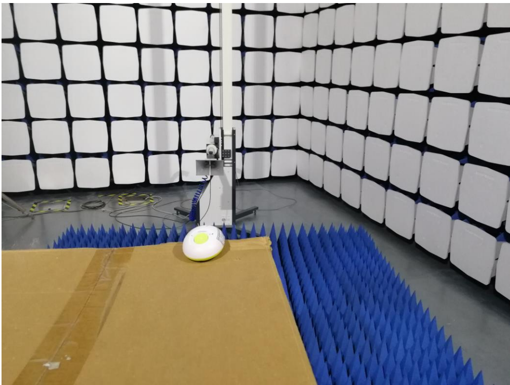
Radiated Emission test view (Frequency above 1GHz)
