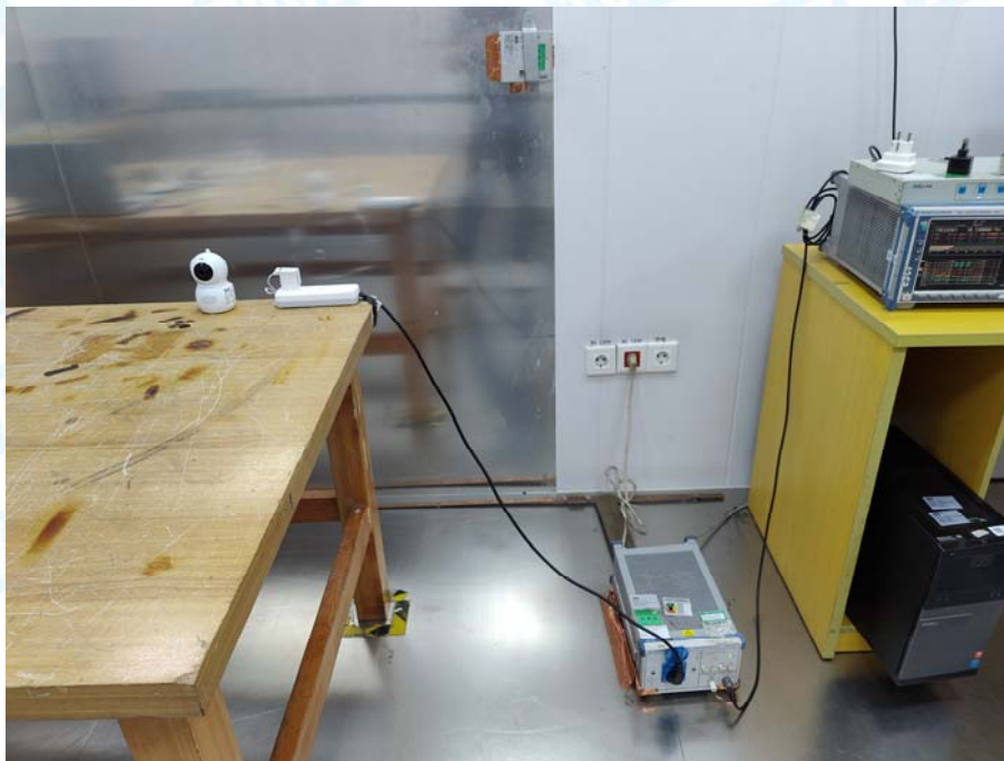
Photo of Setup for Conducted Emission
