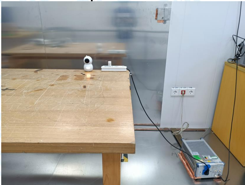
Photo of Setup for Conducted Emission
