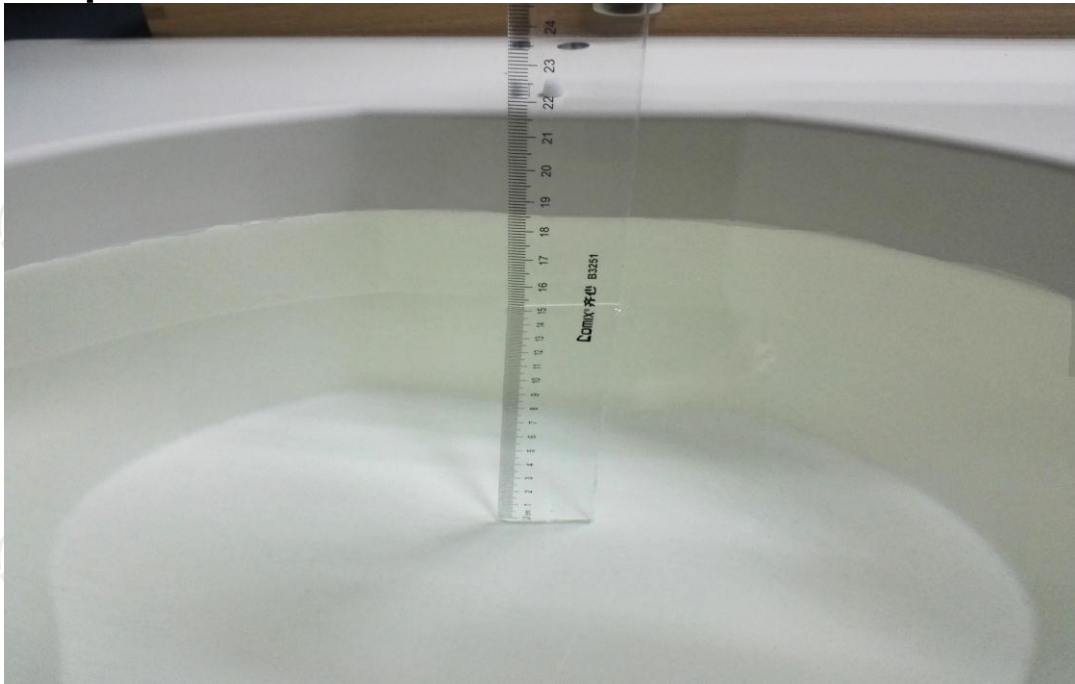
The Body Liquid of 2450MHz (15.3cm)
