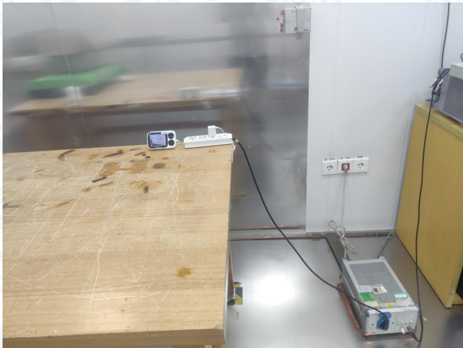
Photo of Setup for Conducted Emission
