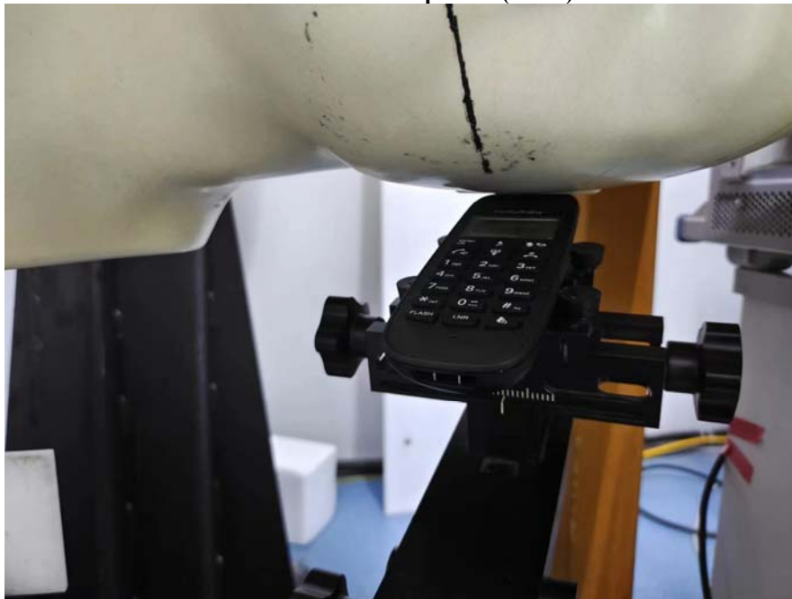
Head Left Tilt Setup Photo(0 mm)
