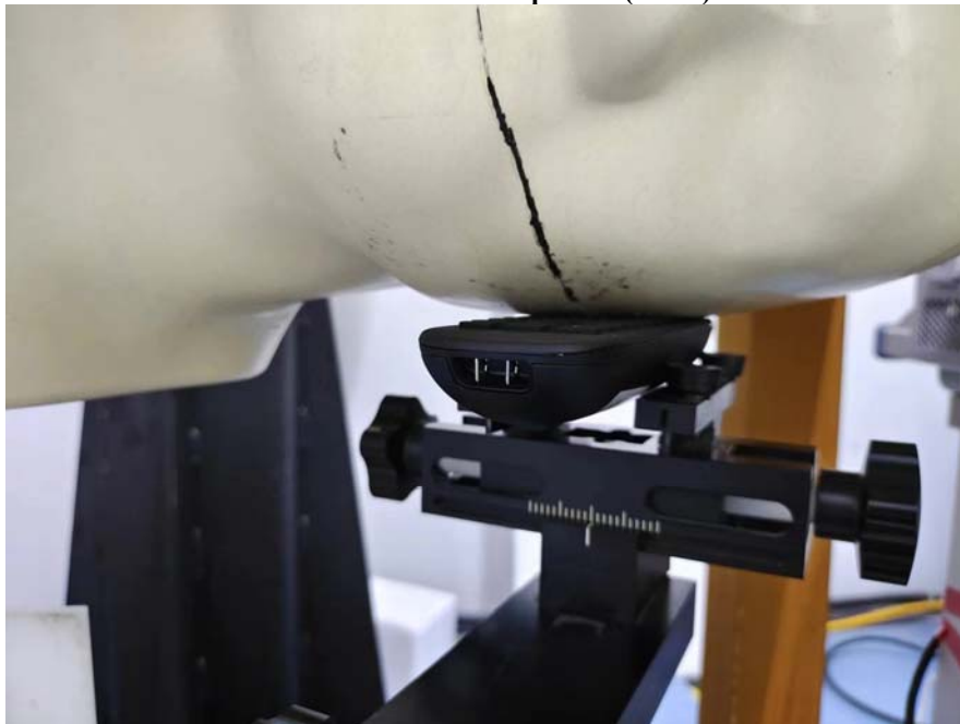
Head Left Cheek Setup Photo(0 mm)
