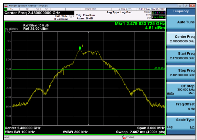
Conducted Emission: GFSK,2480,DH5 ,Reference Level
