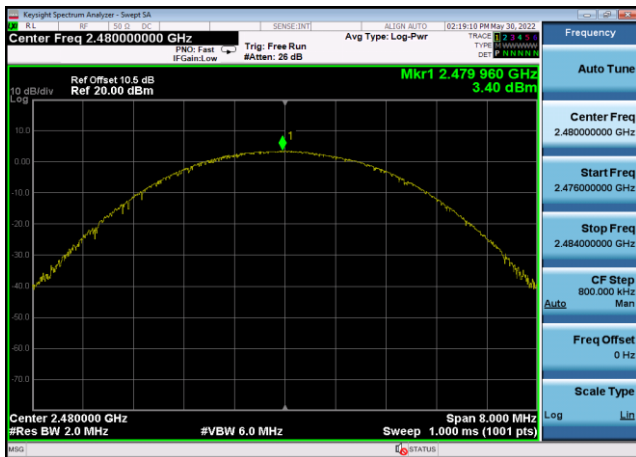
Output Power: 8DPSK,2480MHz,3DH5
