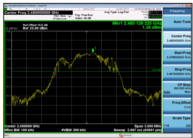
Conducted Emission: DQPSK,2480,2DH5 ,Reference Level
