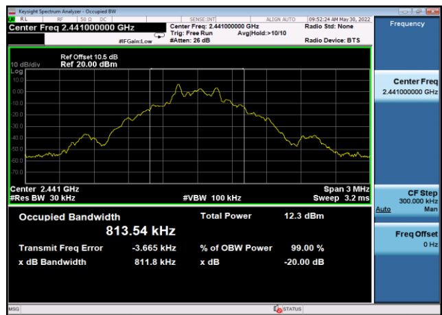
20dB Bandwidth: DQPSK,2402MHz,2DH5
