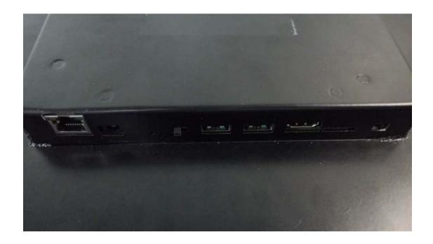
**1.Ethernet:** This interface can provide the function of network data transmission
