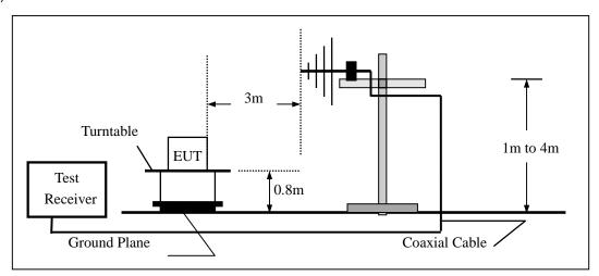
(c) For radiated emissions above 1000MHz
