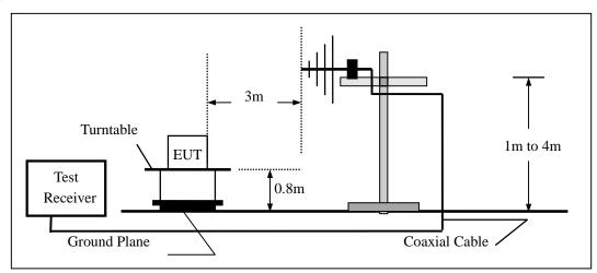
(c) For radiated emissions above 1000MHz
